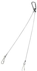
If you anticipate needing to make frequent height and plant proximity adjustments, using a hanging method may be the most optimal solution for you. Secure the two pairs of smaller clips onto the Outer Mounting Holes along the shorter edges of the panel. Then, hook the carabiner onto a suspended system and adjust the height according to your needs.
